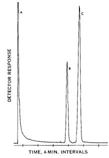
Fig. 1—Chromatogram of U-21699 and lincomycin, A = solvent, B = U-21699, C = lincomycin.
