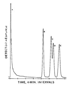
Fig. 3—Chromatogram of lincomycin analogs. A = solvent, B = U-21699, C = lincomycin, D = U-11921. E = U-11973.
