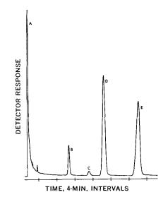
Fig. 2—Chromatogram of an assay preparation from a hard-filled capsule: A = solvent, B = lactose, C =U-21699 and lactose, D = lincomycin, E = internal standard.
